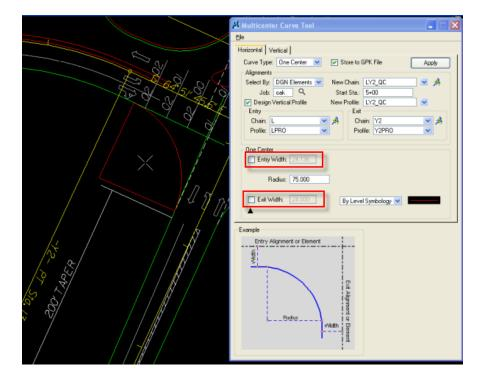
Note about storing the vertical alignment, sometime the proposed TIN file cannot established the entry and exit grade definitions. Try keying-in the proposed super as an option at these key locations instead.
