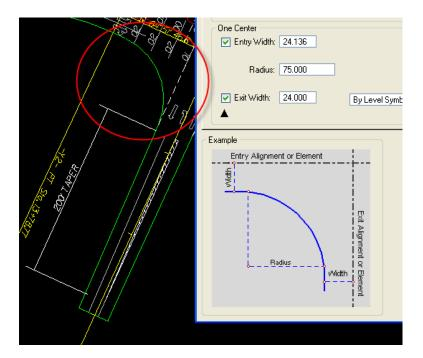
The workaround is to change the Alignment "Select By" method from **GPK Alignment to DGN Element**.
