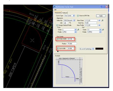
2. Use the EOT graphics (green) to define the entry and exit elements. No entry or exit widths required.
